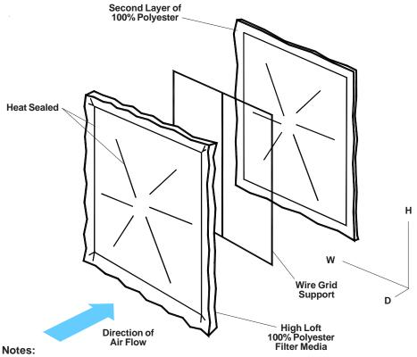
Quality Seal RPDX1 Polyester Ring Panels and RLDX1 Linked Panel Filters are available in 1" thick 2 ply panels. These panels are constructed of a blend of three different fiber deniers in two polyester layers sealed around an internal support wire.
